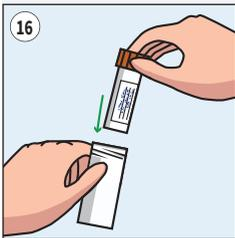
Place SAMPLE tube into the OUTER container keeping the absorbent material between tube and container. Screw the lid onto the outer container.
