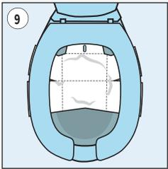
Make sure the EasySampler is taut and in the shape of a bowl. If not, re-orient the flaps for the correct positioning. Lower the toilet seat once the EasySampler is oriented correctly.
