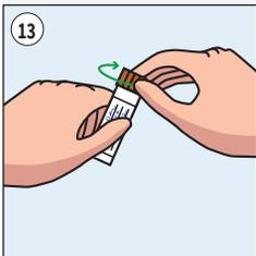
Screw the cap onto the sample tube. A plastic spoon is attached to the brown screw cap for removal of sample at time of testing.
