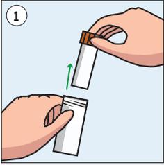
Open the outer container and remove inner sample tube. Leave absorbent material in the outer container.
